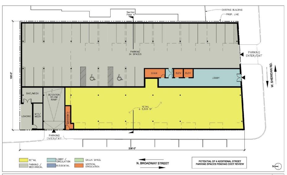
Site Plan/Ground Floor Plan (Parking PI)
