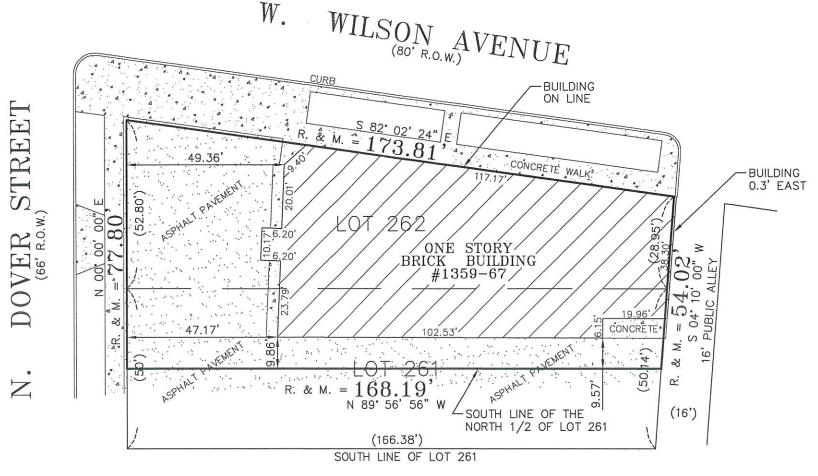
NOTE: R. & M. DENOTES RECORD AND MEASURED DISTANCES RESPECTIVELY BEARINGS SHOWN HEREON ARE MEASURED
